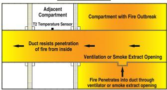
\*DVAC 120 (Non-Coated Fire Rated Ducts) complies with BS 476: PART 24: 1987 and ISO 6944-1 (1985) for 2 Hours Stability & Integrity for Type A & Type B Ducts.
